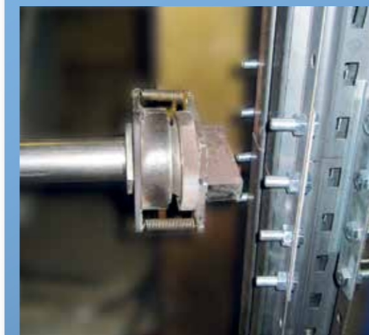
TEST: UPRIGHT SPLICE.
