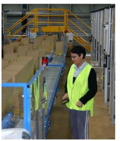
Second best selling lines are in the carton-live storage area, refilled quickly by the replenishment system. The third area has around 4,500 bin picks for the back order catalogue.
