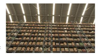
European Manufacturers (FEM), special linking interfaces were used between the racking systems, together with bracing towers every three bays wide. The storage and retrieval machine also meets similar high seismic standards.
